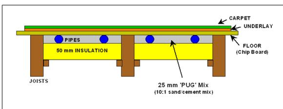
After looking at many options we installed UFH pipes between the joists as shown. We used a dilute 10:1 dry sand / cement 'pug' mix 25 mm thick to spread the heat in preference to heat spreader plates.
