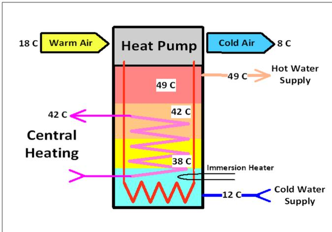
In a Chinese restaurant kitchen there will be plenty of heat where where rice and stir fry are being cooked. At the other end of the kitchen salad may be in preparation and that should be cold. An EAHP can suck in the hot steamy air, take heat out of it to put into hot water for washing up and blow the cooled air into the salad preparation area. An ideal solution!
