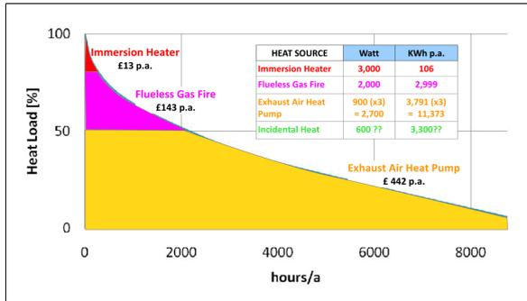
assuming it has a 'coefficient of performance' (COP) of three. I also estimate that there is typically 600 W incidental heat from appliances, solar gain and body heat. This incidental heat is harvested by clever architects, but it makes even a normal house comfortable inside when it is about 15.5 C outside.
