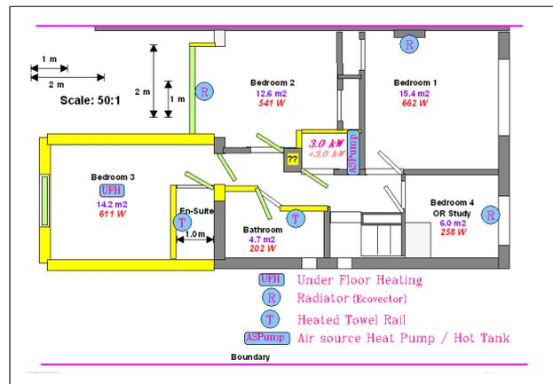
The total heat requirement was calculated from a modified Mitsubishi spreadsheet that can be found at [www.fairshares.co.uk/heating/Heat Loss Calculator.xls](http://www.fairshares.co.uk/heating/Heat Loss Calculator.xls)
